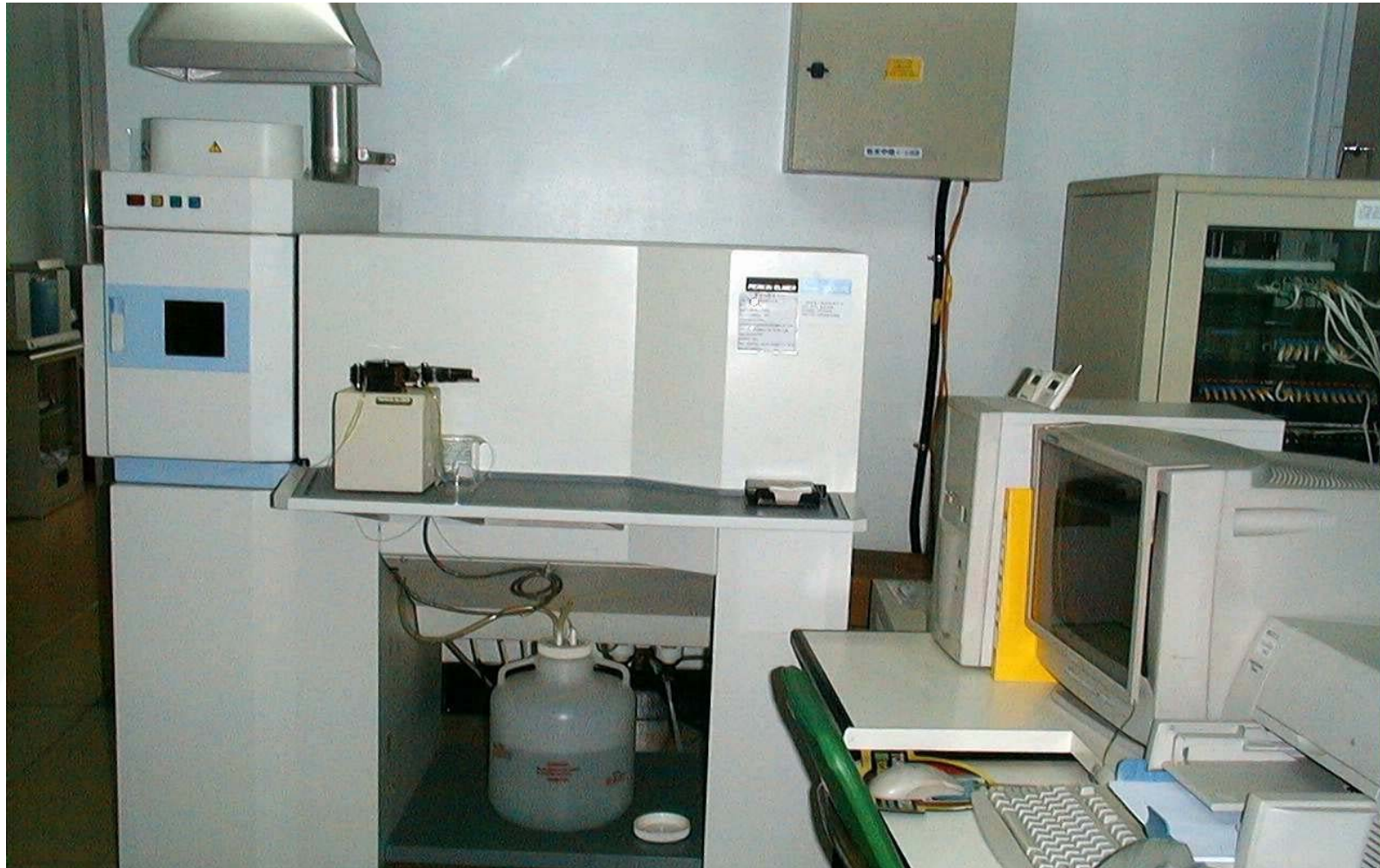
ICP-Emission spectrometry , PERKIN ELMER, OPTIMA 3200L.
