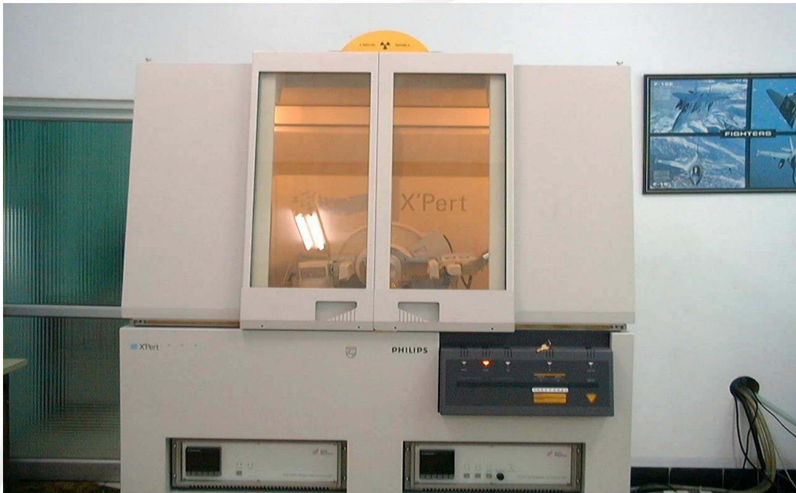
X-ray High temperature and high pressure X-RD analyzer, PHILIPS.
